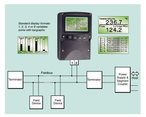
The BA684DF-P Fieldbus Display is a general purpose instrument that can display up to eight fieldbus process variables. Eleven selectable standard screen formats contain one, two, three, four or eight variables, with units of measurement, tag descriptions and bargraphs on some screens.
