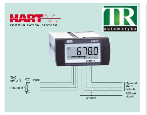
The new BA678C is a second generation panel mounting, loop powered indicating temperature transmitter which replaces the BA578C. It provides an accurate local digital temperature display, plus a 4/20mA output, which may be scaled to represent any temperature range. Although incorporating new facilities such as HART<sup>®</sup> digital communication, diagnostics and a robust enclosure with a IP66 front panel, the BA678C remains electrically compatible with the earlier model.
