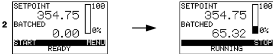
Shows batch setpoint, batched quantity & bargraph depicting batch progress.
