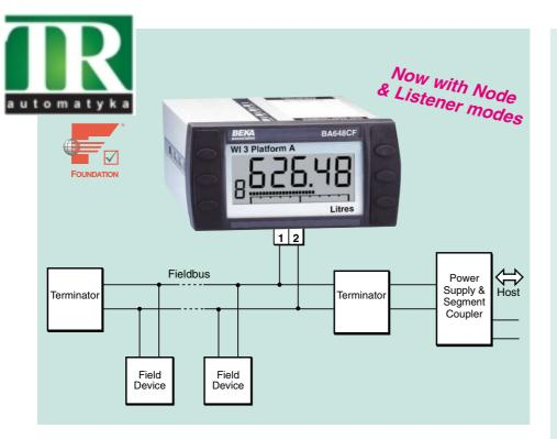
The BA648CF-F Fieldbus Indicator is a general purpose instrument that can display up to eight fieldbus process variables. A numeric annunciator on the left hand side of the screen shows which variable is being displayed. This version of the instrument supports FOUNDATION<sup>™</sup> fieldbus protocol; for PROFIBUS PA systems an alternative version is available – please see the BA648CF-P PROFIBUS datasheet.
