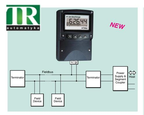
The BA644DF-P PROFIBUS Indicator is a general purpose instrument that can display up to eight fieldbus process variables. A numeric annunciator on the left hand side of the screen shows which variable is being displayed. This version of the indicator supports PROFIBUS PA protocol; for FOUNDATION™ fieldbus systems an alternative version is available − please see the BA644DF-F FOUNDATION™ fieldbus datasheet.
