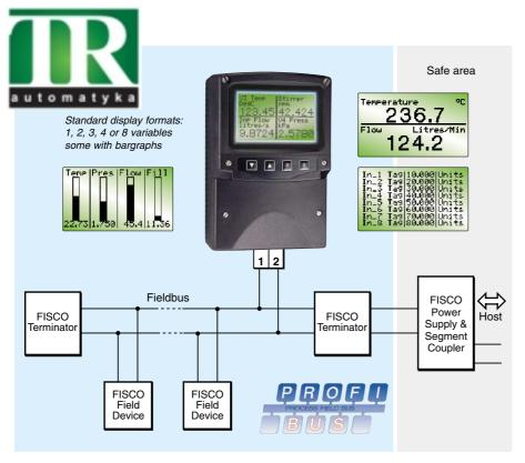
The BA484DF-P Fieldbus Display is an intrinsically safe instrument that can display up to eight fieldbus process variables. Eleven selectable standard screen formats contain one, two, three, four or eight variables, with units of measurement, tag descriptions and bargraphs on some screens.
