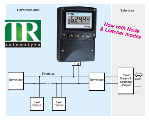
The BA444DF-F FOUNDATION™ fieldbus Indicator is an intrinsically safe instrument that can display up to eight fieldbus process variables within a hazardous area. A numeric annunciator on the left hand side of the screen shows which variable is being displayed. This version of the indicator supports FOUNDATION™ fieldbus protocol; for PROFIBUS PA systems an alternative version is available – please see the BA444DF-P PROFIBUS datasheet.
