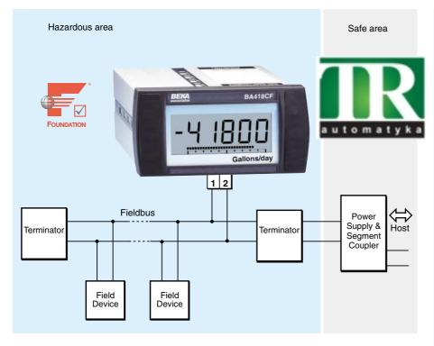
The BA418CF-F Fieldbus Indicator is a new cost-effective intrinsically safe panel mounting instrument that displays a single fieldbus process variable in a hazardous area. Housed in a robust panel mounting enclosure with an IP66 front, the instrument has a large, high contrast five digit display and a horizontal bargraph. The BA418CF-F indicator uses the same technology and compliments the well established BEKA eight variable fieldbus displays that are now in worldwide use.
