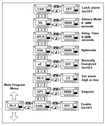
**8.6.6)** "dELA" - Delay. This function can be programmed to delay alarm activation by up to 3600 seconds. If set to "0000" then there is no delay in the alarm.
