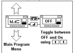
Normal Display Mode with this parameter set to "On", the maximum and minimum temperatures can be displayed (by pressing the up and down buttons) and reset (by pressing up and down buttons together). The maximum and minimum temperatures will be lost if there is a power failure.
