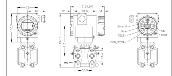
\* without display and operating module marked dimensions decrease by 19 mm
