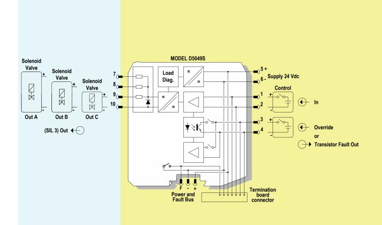
Terminals 3-4 dip-switch selectable for fault output signaling or override control
