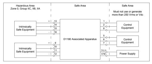
Tamb -20 to +60 °C, and connected to equipment with a maximum limit for AC power supply Um of 250 Vrms.
